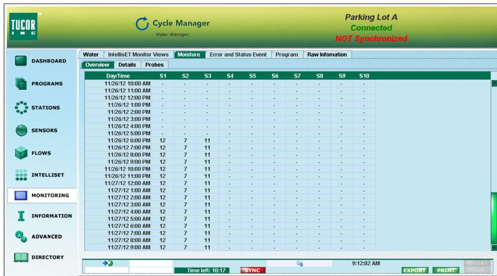
**Figure 4:** The **Overview** subtab provides basic information about sensors and probes.
