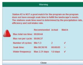
This warning tells that there is not enough soak time. This may be due to the fact that the system sets the end time so that the two cycles are run in succession.
