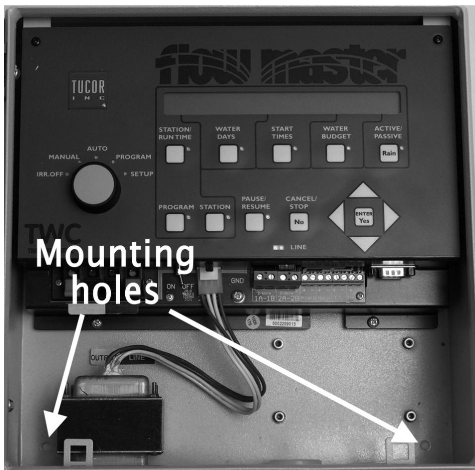
5. If you're placing the controller on a concrete wall, take down the controller, drill out the holes for the two new screws, possibly put in the wall anchors, and put back the controller on the wall.
