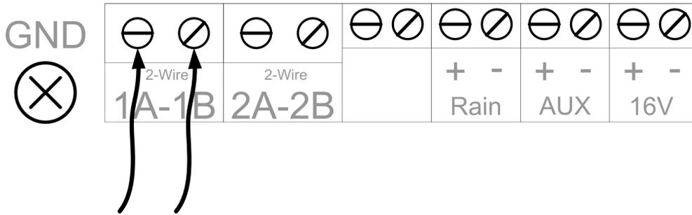
There's room for connecting two cables directly to the controller - the other line can be connected to the terminals labeled 2A-2B. Both wires will receive the same signals when the controller is up and running.
