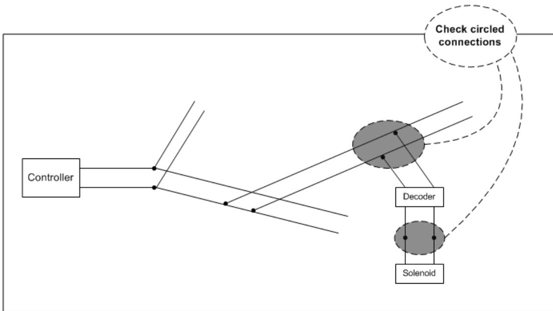
**Figure 7.2. Testing the path to a decoder**
